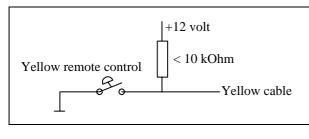
The yellow cable is meant to be connected to the reverse light as default to reverse counting when the vehicle is reversed. However for a rallycar it is more convenient to use it as a second remote control (See page 25). For this reason the remote control for the yellow
