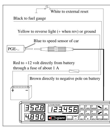
Make sure all connections are done professionally. The cables should be fixed to avoid damage. Most disturbances in function that occur are caused by poor connections to the power supply. After having carried out these functions
